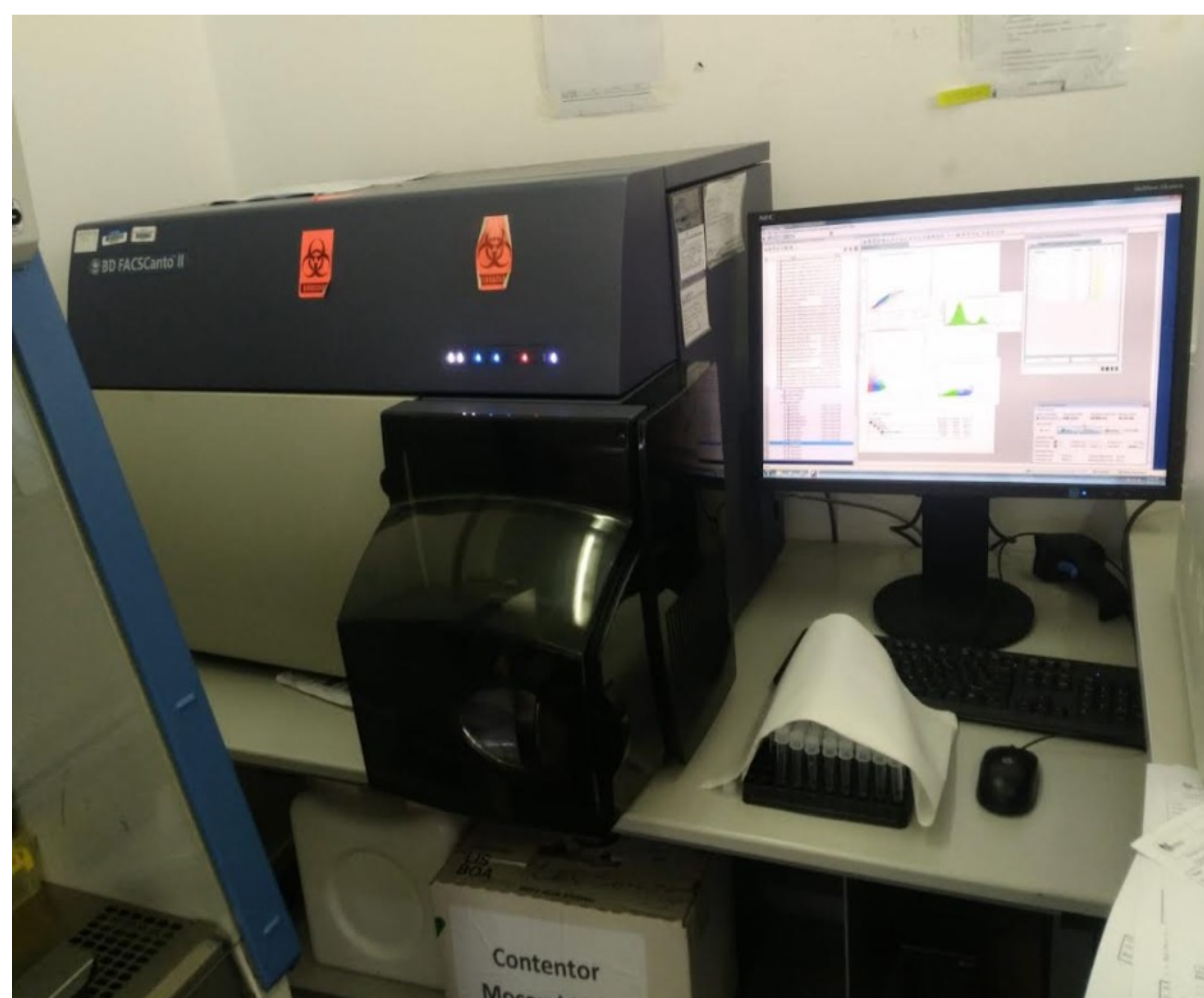
Figure 1: BD FACSanto II used for flow cytometric differential diagnosis of leukaemia
